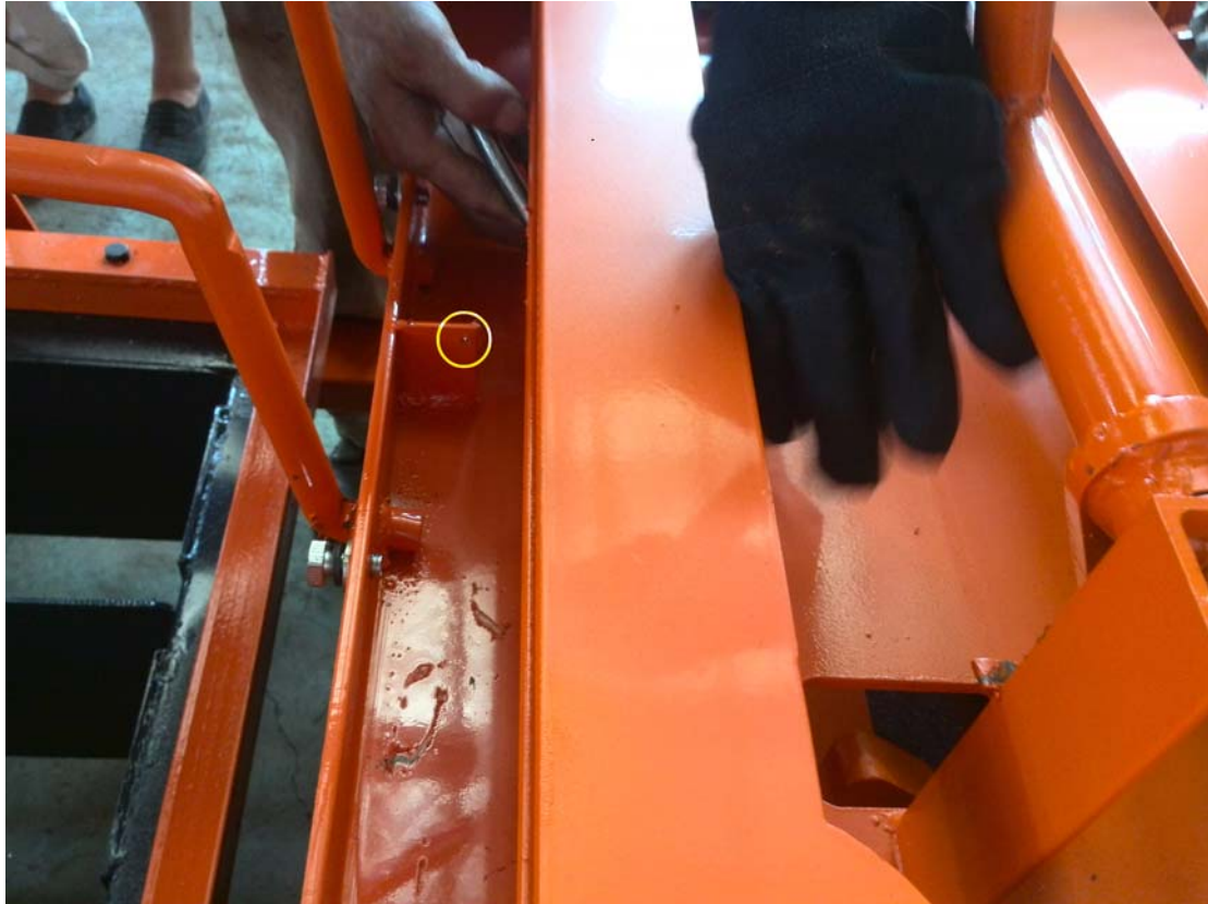
The other side of spring hooks the hole of steel plate.
