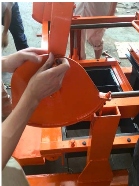
Lower mould lifting system(handle with counterweight at both sides)
