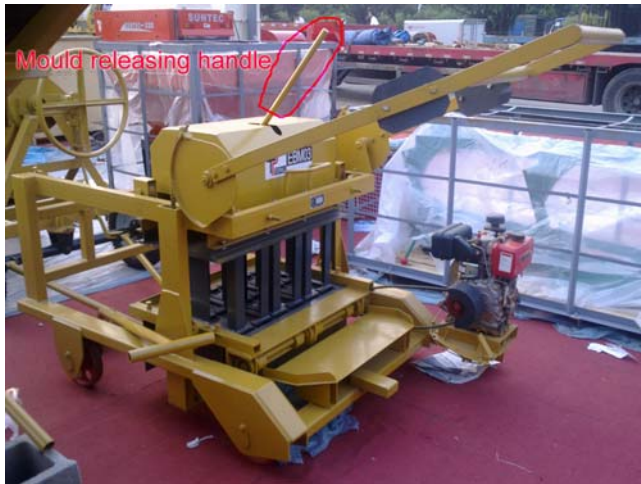
Lower mould lifting system(handle with counterweight at both sides)
